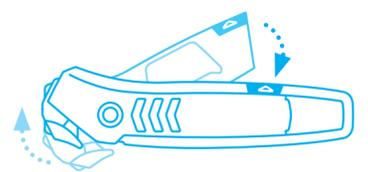
Push the blade magazine **back into the handle** to lock the blade head in place.
