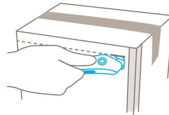
Use the nose of the cutter to **pierce** into the cutting material. **Do not lever** against staples, nor force the nose into edge protectors!
