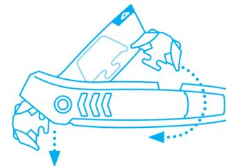
Remove the fitted blade from the head of the cutter. Now you can either **rotate or replace** the blade.
