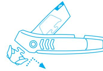
Position the spare blade **parallel** to the slanted side of the cutter head. Push the blade in, and then **downwards**, until fully engaged.
